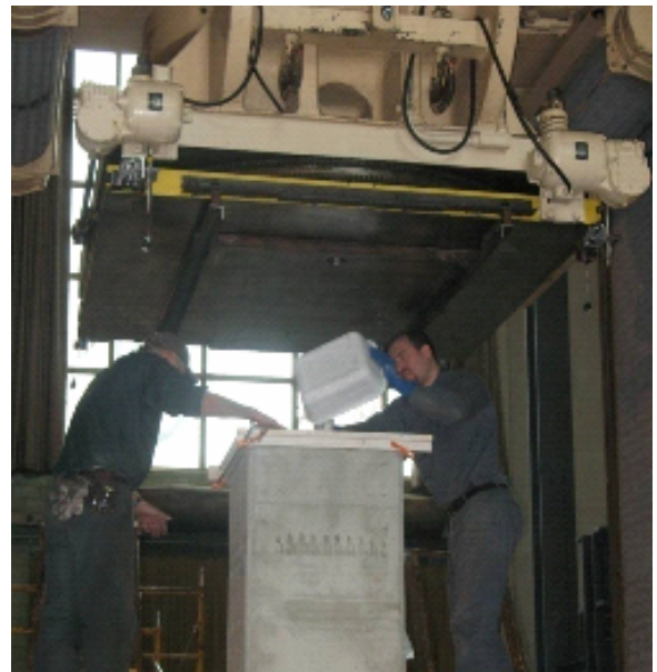
Figure 10 – Hydro-stoning of the top surface
