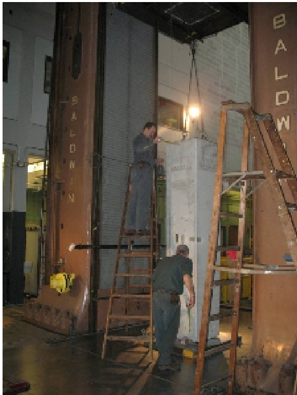
Figure 8 – Column specimen centered and plumbed
