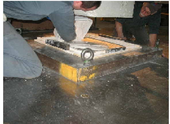
Figure 9 – Hydro-stoning of the bottom surface
