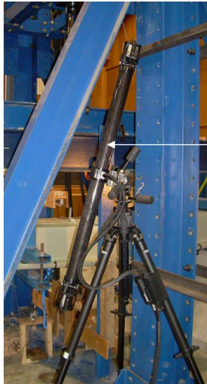
**Figure 11. Non Contact Optical 3D Measuring System. Pontos.**
