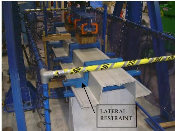
**Figure 9. Four-Point Bending Sheet piling Testing Set-up**
