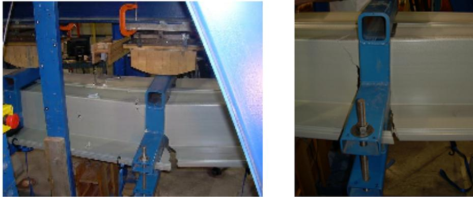
Figure 13. WPC Sheet Piling Shear Failure.
