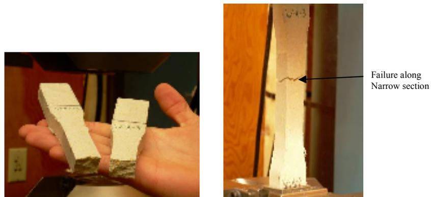
**Figure 8. WPC Specimen Tension Failure.**
