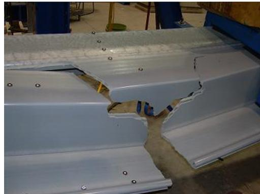
**Figure 12. WPC Sheet Piling Tensile Failure.**
