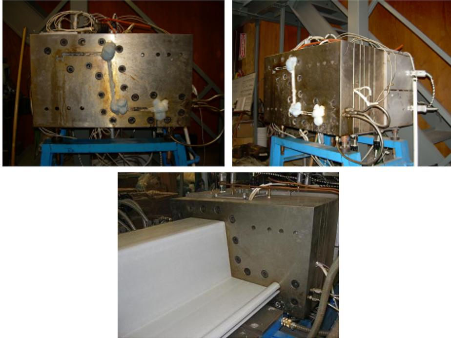
**Figure 3. WPC Z-Section Extrusion Die**
