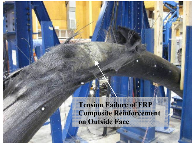
Figure 8. Arch Secondary Failure Mode
