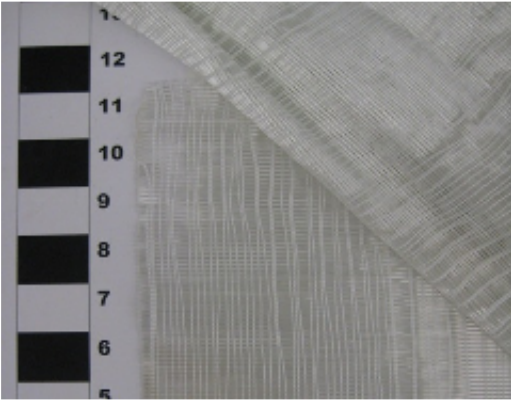
Figure 1 - S560, low density glass fiber sheet (inch scale).
