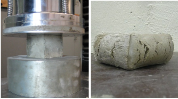
Figure 12 - Compression failure of grout type-A.
