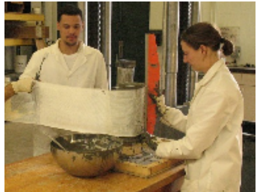
Figure 5 - Knife edge and start of fiber wrapping.
